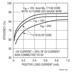
Figure 3. Dual Output Efficiency
